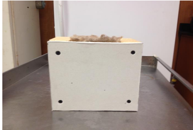
Figure 2.3 Picture of the interior side of the residential building wall showing the gypsum wallboard.
