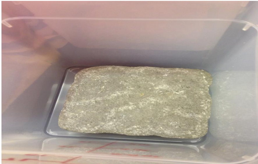
Figure 2.6 Paver stone at the bottom of the mold chamber The wall sat on top of the paver stone during the study.
